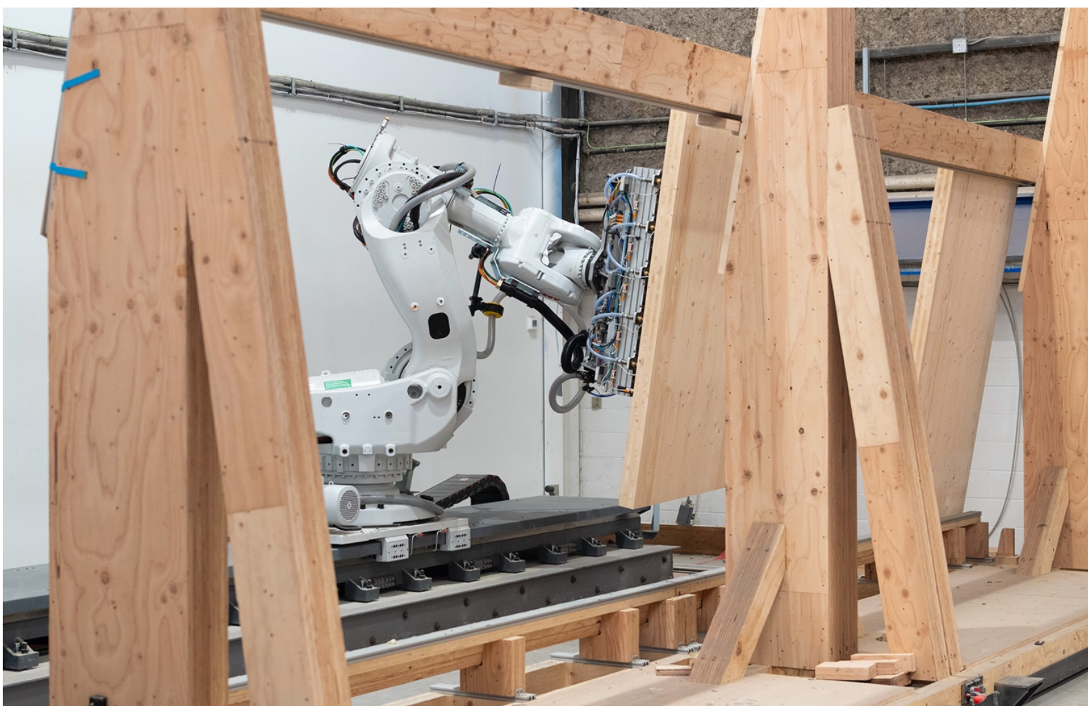
Automated mass timber panel fabrication at Intelligent City, Vancouver (image credit: Intelligent City).
