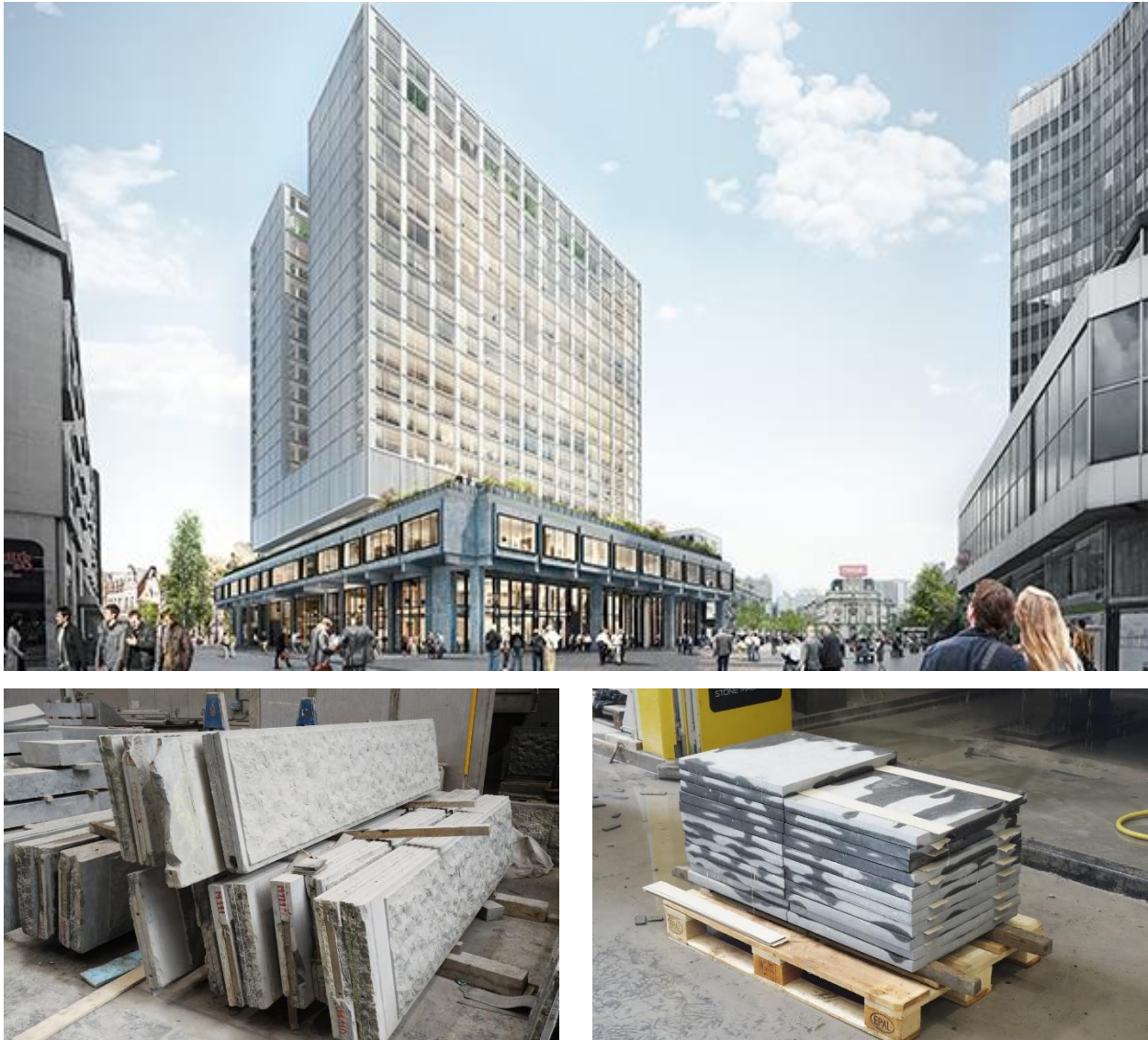
Figure 15: Multi project, Brussels (top) with the salvaged limestone panels (bottom left) that were reprocessed into paving slabs (bottom right). Photo credit: Rotor Deconstruction
